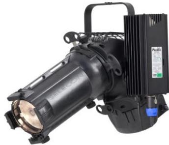
**The original 80V Power Supply is an electronic transformer tracking the incoming (dimmed) supply to deliver a maximum of 80V at the lamp. Mains supply input 220V-240V to be supplied via a high quality entertainment type dimmer. The transformer output tracks the dimmer output, typically the response delay is as experienced with 2000W mains voltage luminaires.**
